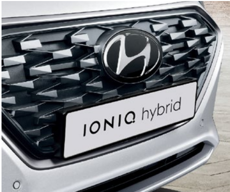
Front grille The IONIQ Hybrid & Plug-In's floating three-dimensional mesh-type grille features computer-controlled shutters that open and close automatically to improve aerodynamics.
