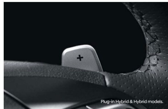
Paddle Shifters - Transmission control or regenerative braking control
